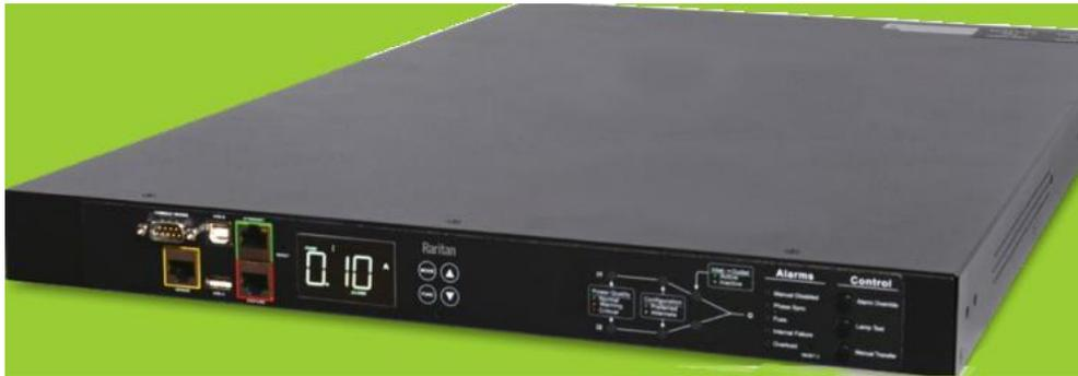
The PX3TS transfer switch provides AC power to rack IT equipment from one of two AC power sources, and automatically selects which source powers the load based on power availability and quality.
