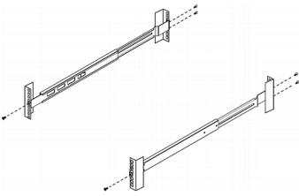
3. Line up the mounting brackets with slide-rails and push this product into rails.
