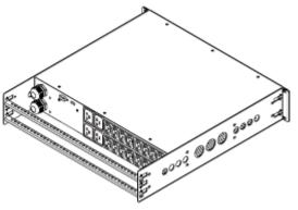
Fasten the rackmount brackets' ears to the rack using your own fasteners.
