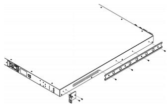
2. Adjust slide-rail assemblies to match your rack posts and fasten them to the rack using your own fasteners.
