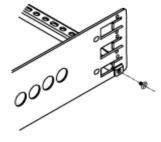
On a 2U model, repeat the above steps to install another cable-support bar.
