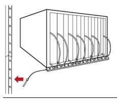
Note: If you need to temporarily disconnect the blade extension strip from the asset strip, wait at least 1 second before re-connecting it back, or the managing device may not detect it.
