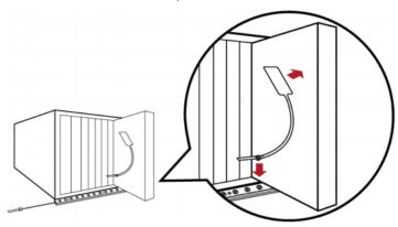
4. Repeat the above step until all blade servers in the chassis are connected to the blade extension strip via asset tags.
