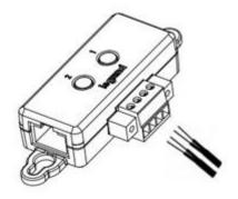
3) Use a screwdriver with a 2.5 mm wide shaft to tighten the screws above each termination point to secure the wires, using a torque of 0.196 N·m (2 kgf·cm).
