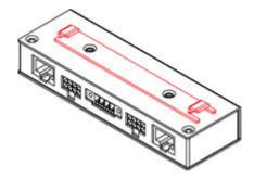
► Bracket installed onto the side of DX2-DH2C2:
