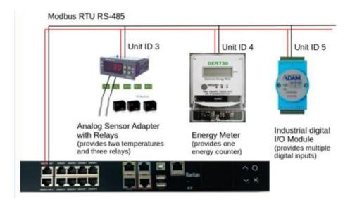
To connect external sensors to all Xerus-firmware devices USB-A with USB-MODBUS-DONGLE:
