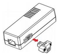
3) After connecting detectors/switches to the terminal module, plug the terminal module back into the sensor box, and then tighten the screws at two sides of the terminal module.
