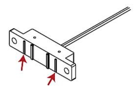
When water is present between the 2 poles, the water sensor will trigger the alarm.
