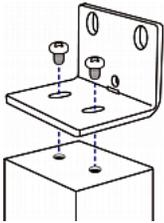
2. Choose either of the following ways to fasten the PDU to the rack.
