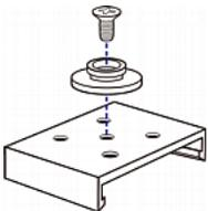
4. Fasten the device to the rack or cabinet using the baseplate-based tools.
