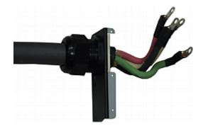
Temporarily hand tighten the gland nut and verify the cord cannot be twisted or pushed or pulled in the gland. Do not proceed if hand tightening results in a loose cord. In some models, especially in-line monitors, the flexible cord's diameter may be too small for the cable gland. A sealing ring for smaller diameter line cords may have been included with the Raritan product, or can be requested from Raritan, to reduce the inside diameter of the cable gland.
