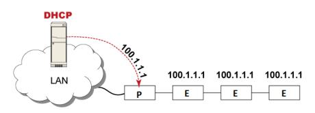
*In this mode, the DHCP server communicates with the primary device alone and assigns one IP address to the primary device. All expansion devices share the same IP address as the primary device.*
