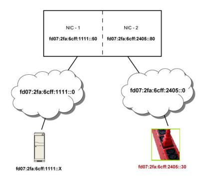
In this example, NIC-2 (fd07:2fa:6cff:2405::80) is the next hop router for your PX-Series PDU to communicate with any device in the other subnet fd07:2fa:6cff:1111::0.
