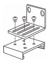
5. Using rack screws, fasten the device to the rack through the L-brackets.
