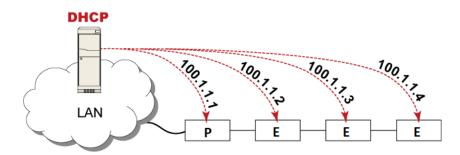
In this mode, the DHCP server communicates with every cascaded device respectively and assigns four different IP addresses. Each device has its own IP address.
