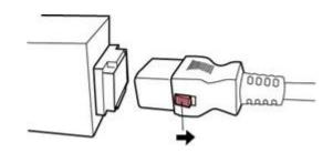
Installing Cable Retention Clips on the Inlet (Optional)
