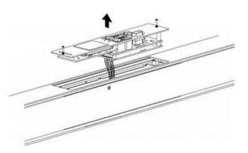
3. Disconnect the PDU's controller cable from the controller.
