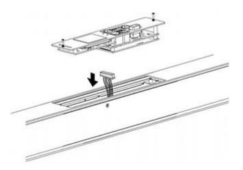
4. Get a new controller and install it back into the PDU in the reverse order.
