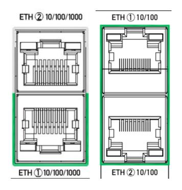
Warning: Accidentally plugging an RS-232 RJ-45 connector into the Ethernet port can cause permanent damage(s) to the Ethernet hardware.
