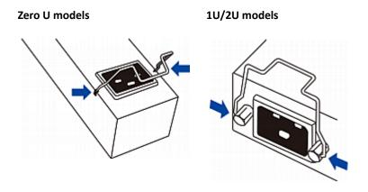
3. Connect the power cord to the inlet, and press the clip toward the power cord until it holds the cord firmly.
