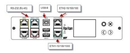
To use the command line interface (CLI) for configuration, establish an RS-232 or USB connection.
