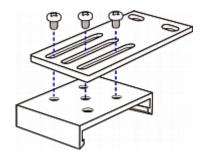
5. Using rack screws, fasten the device to the rack through the claw-foot brackets.
