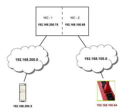
In this example, NIC-2 (192.168.100.88) is the next hop router for your PX-Series PDU to communicate with any device in the other subnet 192.168.200.0.
