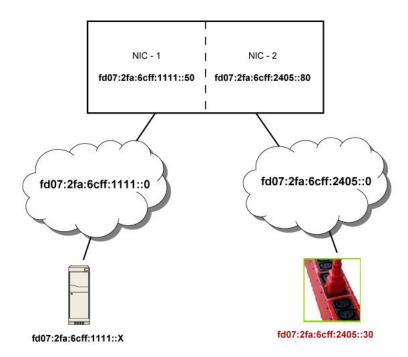
In this example, NIC-2 (fd07:2fa:6cff:2405::80) is the next hop router for your Legrand PDU to communicate with any device in the other subnet fd07:2fa:6cff:1111::0.
