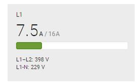
The right side shows the current and voltage data per phase. For a single-phase device, it shows only one line, but for a three-phase device, it shows three lines (L1, L2 and L3).
