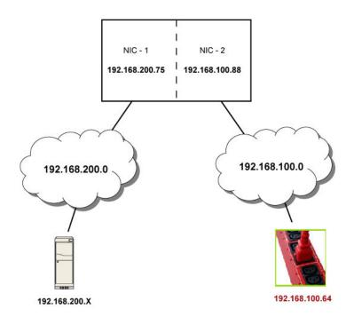
In this example, NIC-2 (192.168.100.88) is the next hop router for your Legrand PDU to communicate with any device in the other subnet 192.168.200.0.
